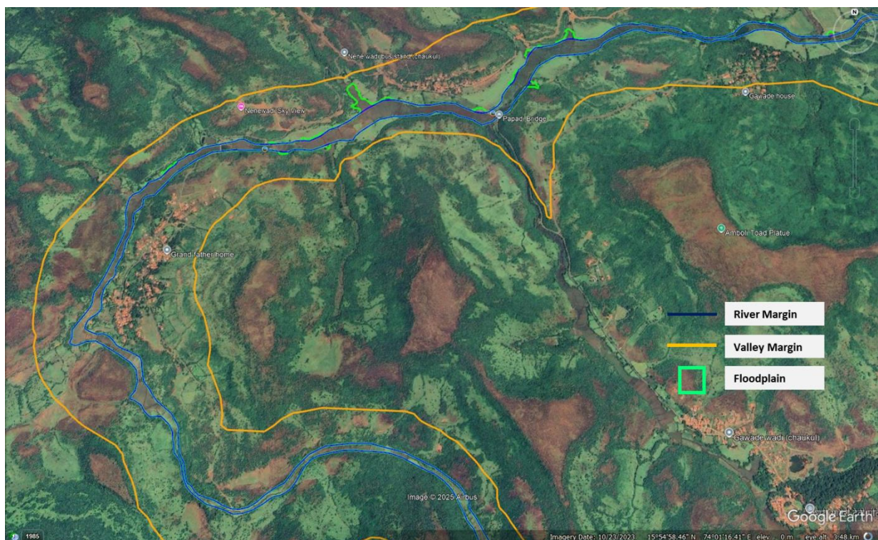
Figure 7. 17 Partly confined, discontinuous bedrock–floodplain system with gorge sections and a boulder-bed channel in the Upper Krishna
