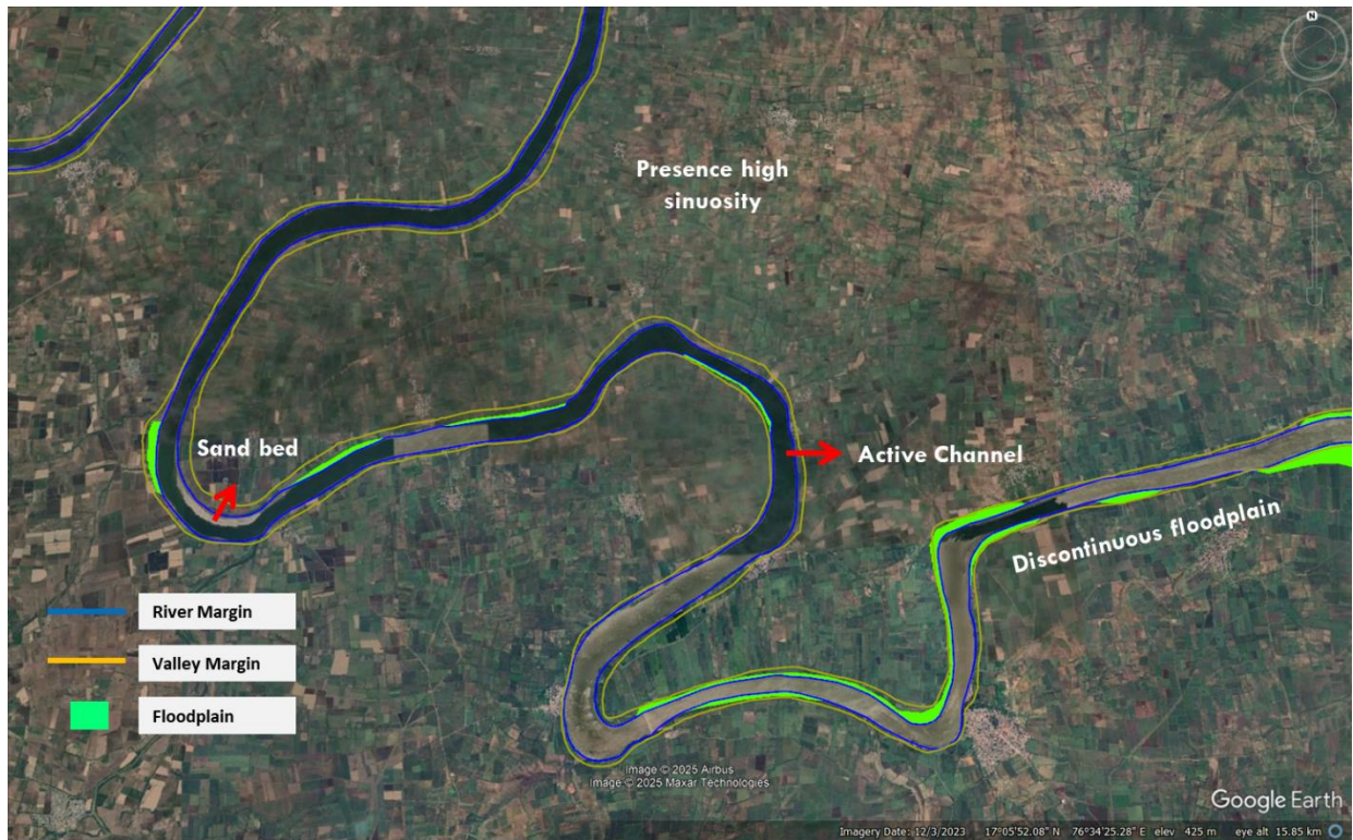
Figure 7. 8 Partly confined, planform-controlled, discontinuous floodplain with a high-sinuosity sand-bed channel in the Lower Bhima sub-basin
